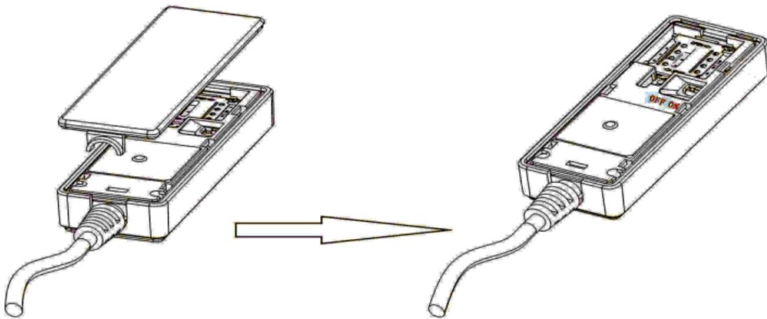
2.1.4 Switch device must be switched to "ON" when using, as shown.
